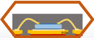
Wire bond at lead frame or substrate
