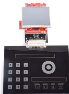
BLE & Capacitive Touch Control Panel Solution
