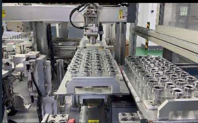
Automated Inspection OAD Shaft
