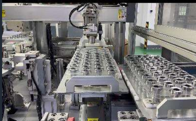
Automated Inspection OAD Shaft
