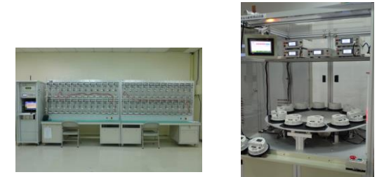
Insulation withstand voltage testing device
