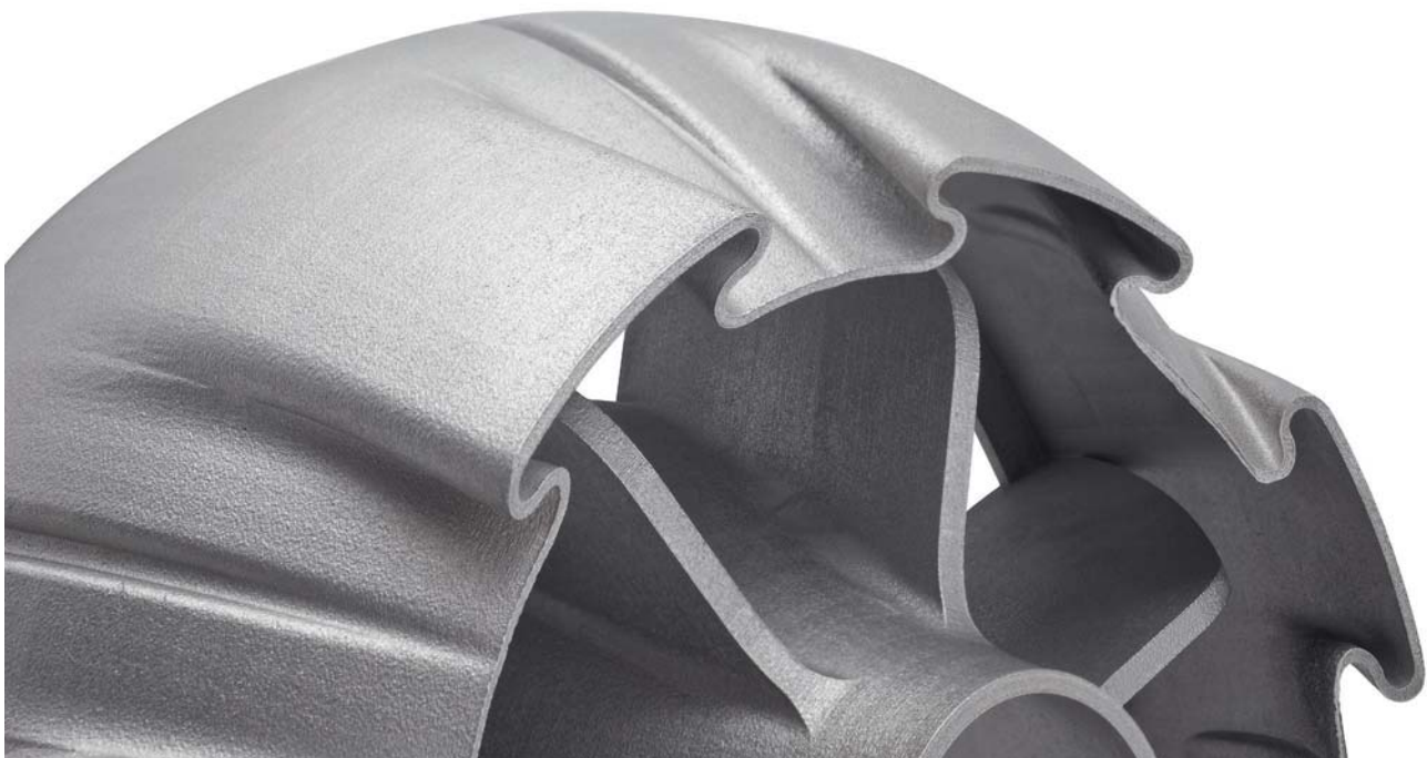
Above: A demonstration component typical of those used for modelling flow dynamics of a turbine produced using a Renishaw laser melting machine
