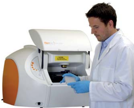
Above: RA800 series benchtop Raman instrument
