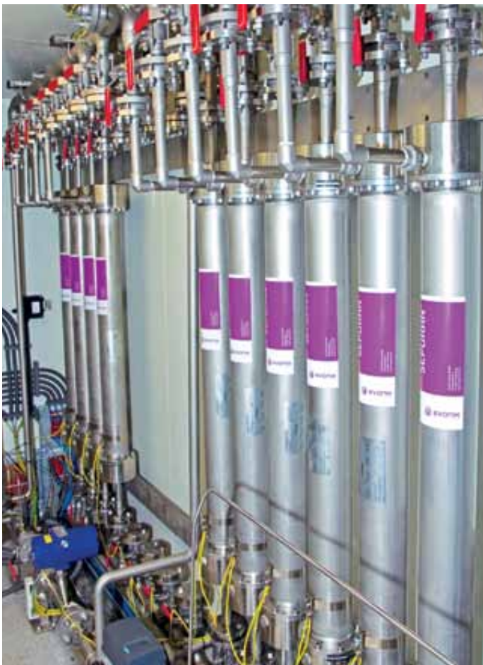
In rank and file: Interior view of the plant with SEPURAN® Green membrane modules.
