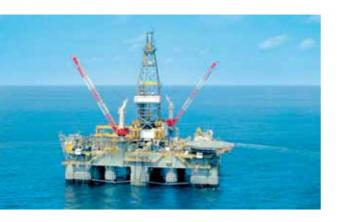
HCI Deepsea Oil Explorer is equipped for drilling at depths of up to 2,400 metres.
