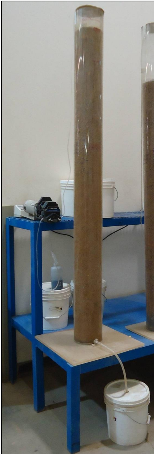
Figure 6-2. ODAS/Stratex Project Column Leach Test Apparatus
