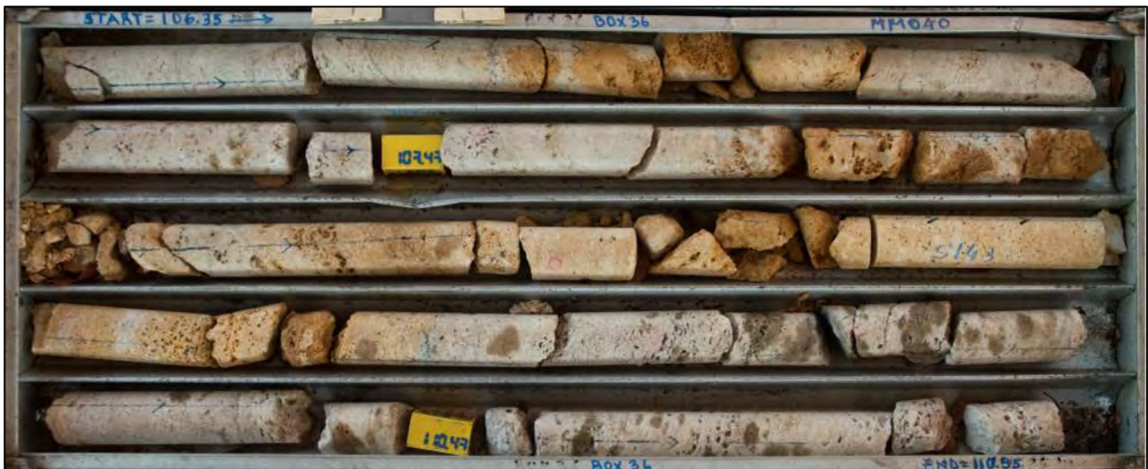
Figure 4.39 MM040 box 36 106.35 to 110.95 m showing typical void presentation
