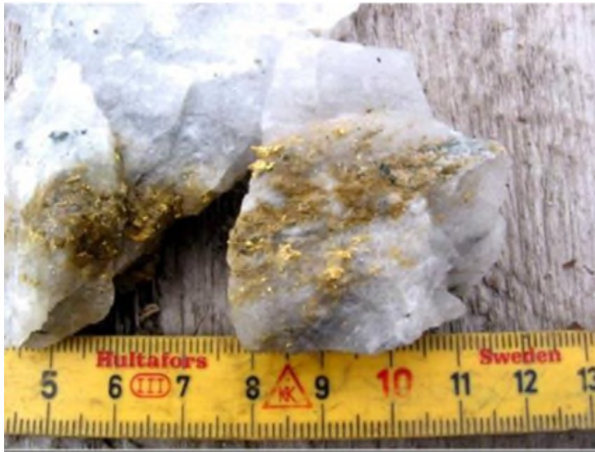
Figure N-10 High grade gold-quartz vein sample from the Nalunaq Main Vein containing coarse gold (source: Crew Gold).
