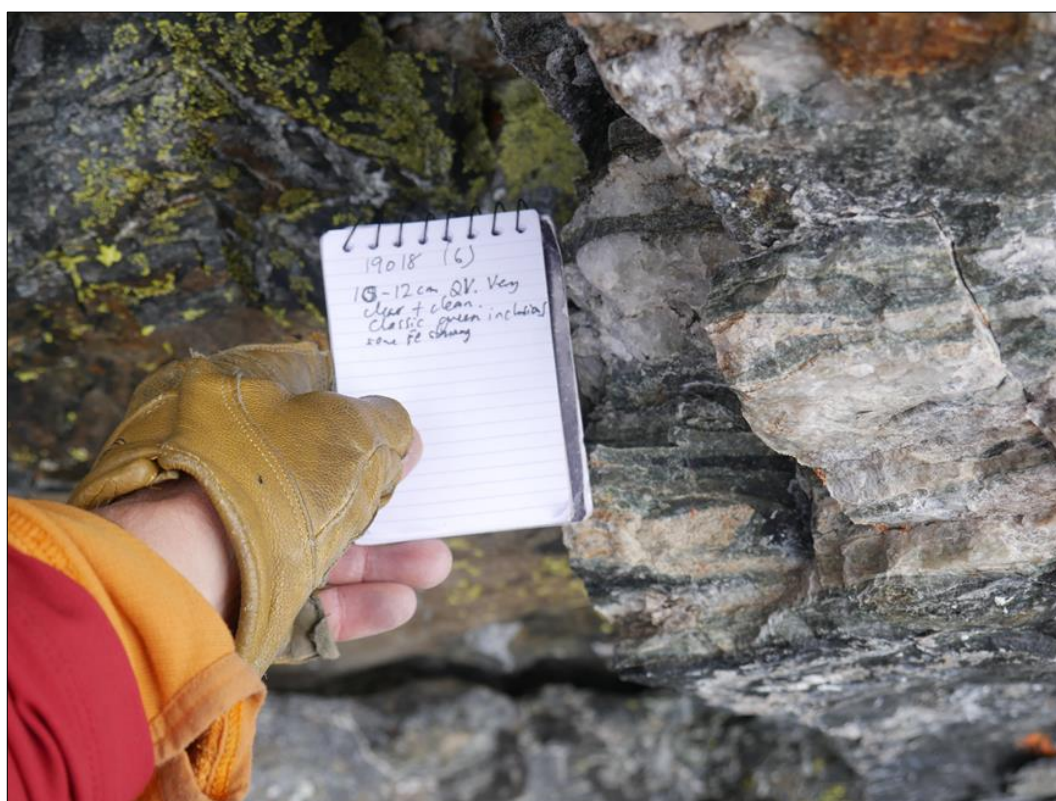
Figure 6-5: Sample 19018 quartz veining surrounded by calc silicate alteration assaying 2.1 g/t Au
