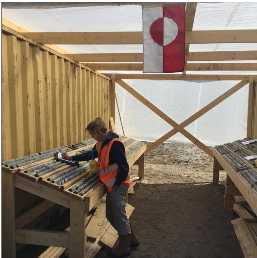
Figure 5-18: Core logging at Nalunaq in 2017 (AEX, 2017)
