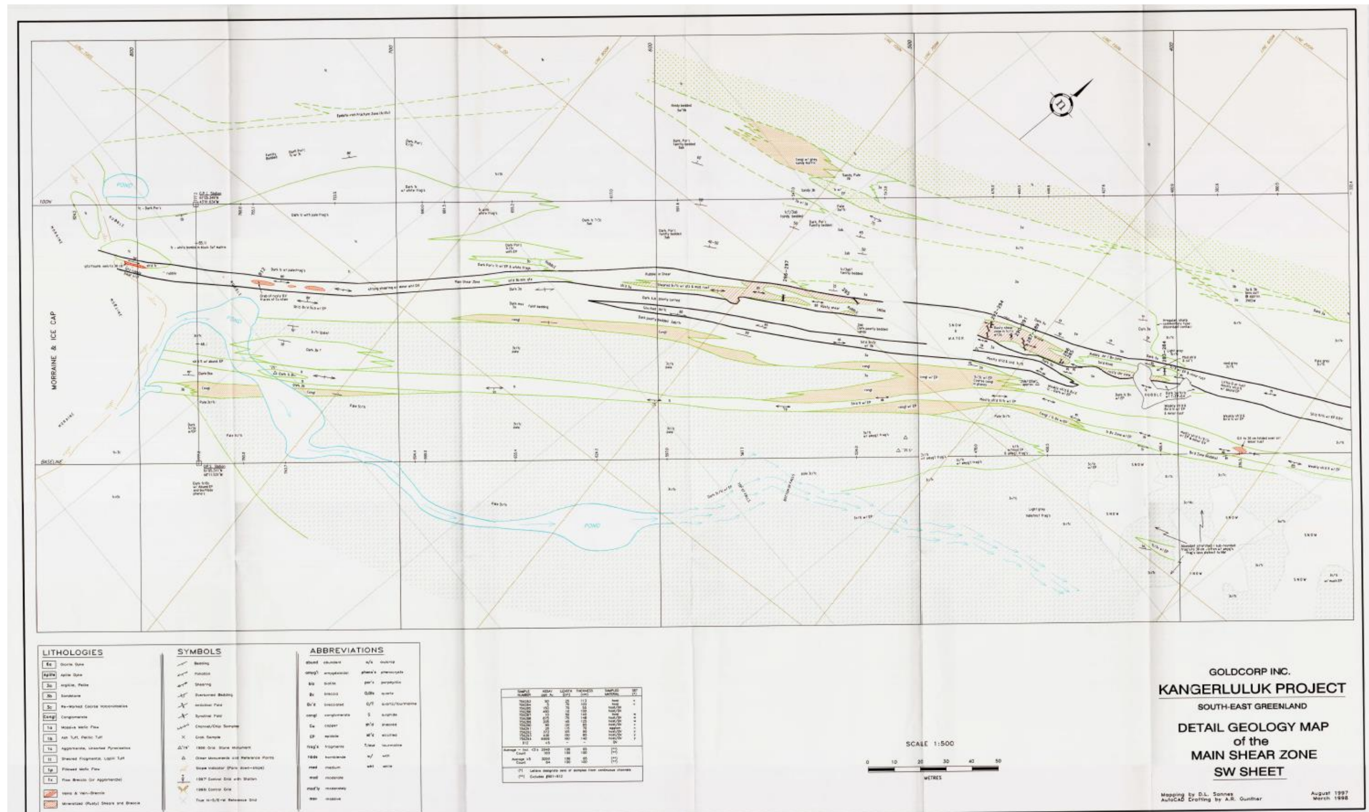
Figure 8-10: Geological map of the main shear zone, SW section, Kangerluluk, showing Goldcorp channel sample locations (Sannes, 1998)
