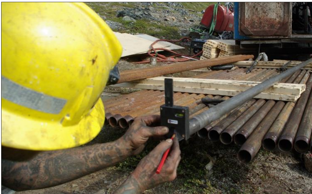
Figure 5-15: Marking the bottom of hole line on drill core using the Reflex ACT tool in 2017 (AEX, 2017)
