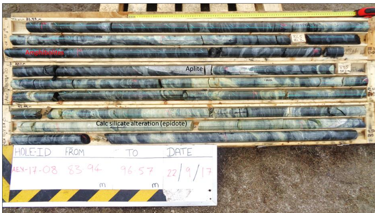
Figure 5-20: Example of the typical lithologies and alteration intersected during drilling at Nalunaq (AEX, 2017)
