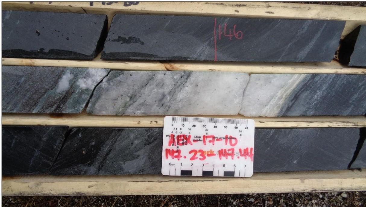
Figure 5-5: Quartz vein containing visible gold interpreted to be MV from drill hole AEX1710 at 147.23 - 147.44 m (AEX, 2017)
