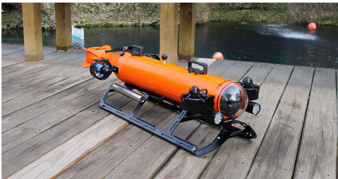
Aquabotix's second-generation hybrid vehicle, the Integra AUV/ROV
