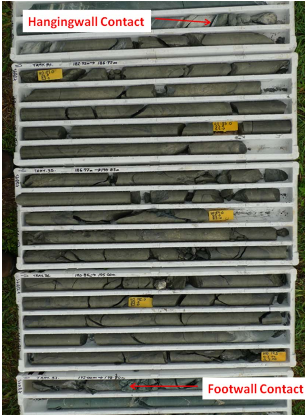
Figure 1 – Mineralised interval from hole FRWD0002 - 13.5m (11m TW) @ 3.3%Cu, 4% Zn and 30g/t Ag
