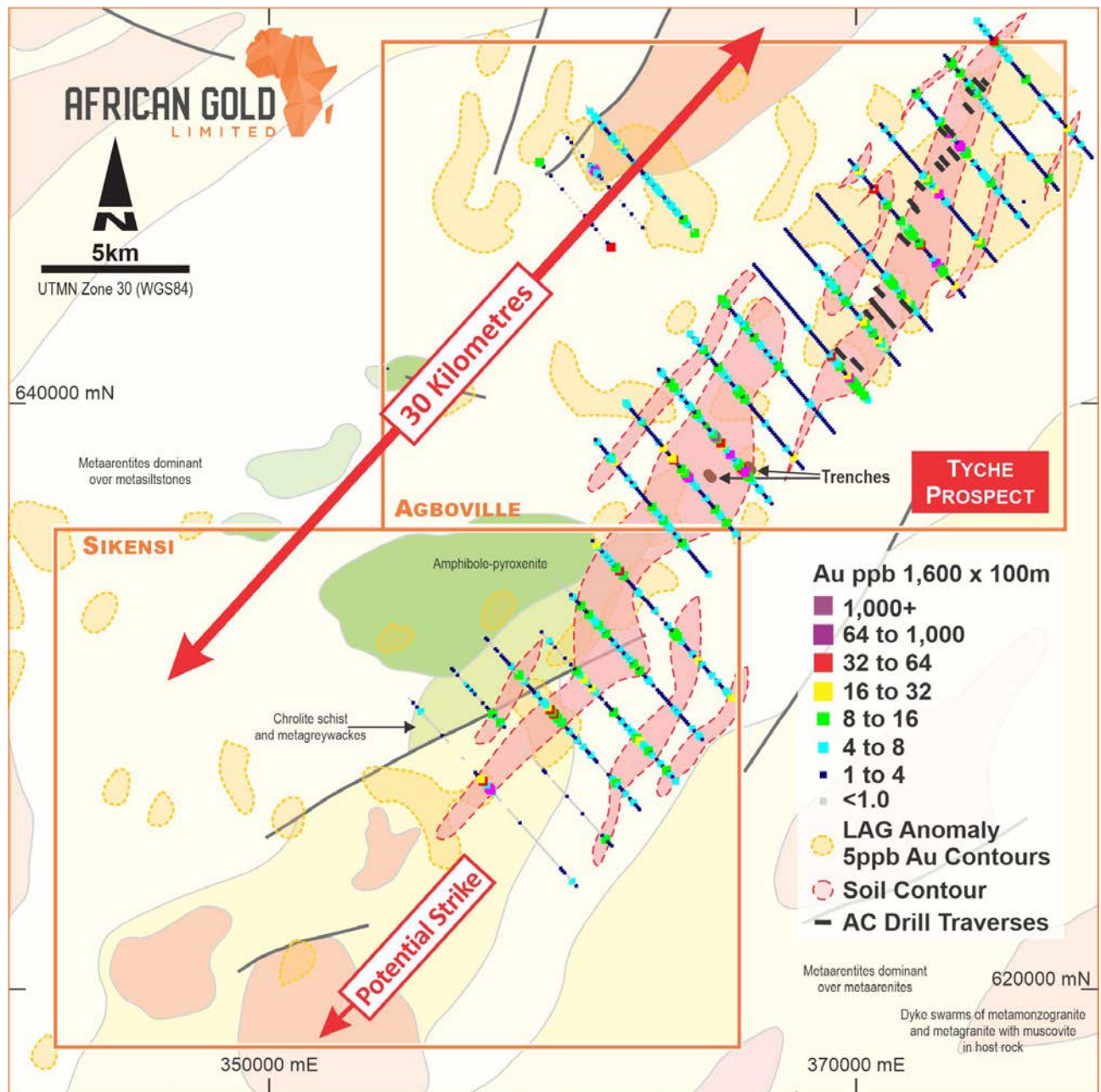
Figure 7: Agboville Project – Tyche Gold Prospect, thematically mapped gold on simplified geology, also showing lag anomalies, location of drilling and location of contoured gold-in-soil anomaly and location of Aircore drill traverse completed in April-May 2019 and trenches completed August 2019.
