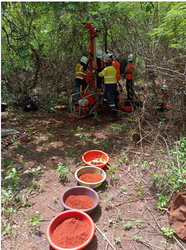
Figure 2: Auger drilling at Konahiri North Gold Project
