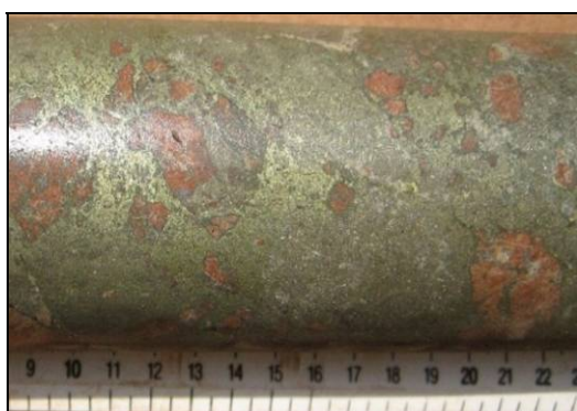
Semi-massive chalcopyrite in altered syenite (KITDD_008, 520 m)
