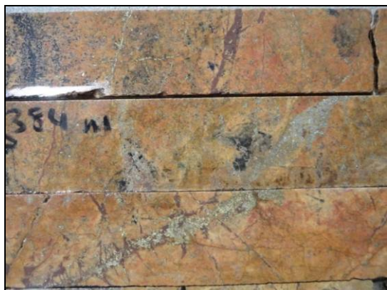
Fracture-hosted pyrite \pm chalcopyrite in carbonate-altered syenite (S36-033, 384 m)
