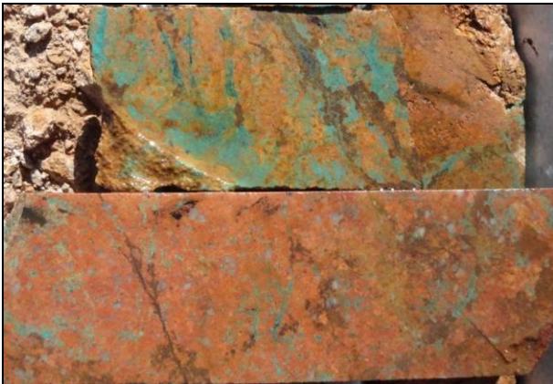
Malachite and pseudomalachite along fractures in quartz porphyry granite (S36-001; 126 m)
