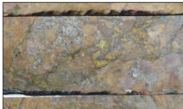
Fracture-hosted pyrite and chalcopyrite in altered syenite (S36-033, 413 m)
