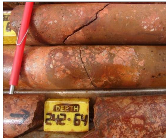
B) Potassic alteration partially overprinted by hematite alteration (S36-001)
