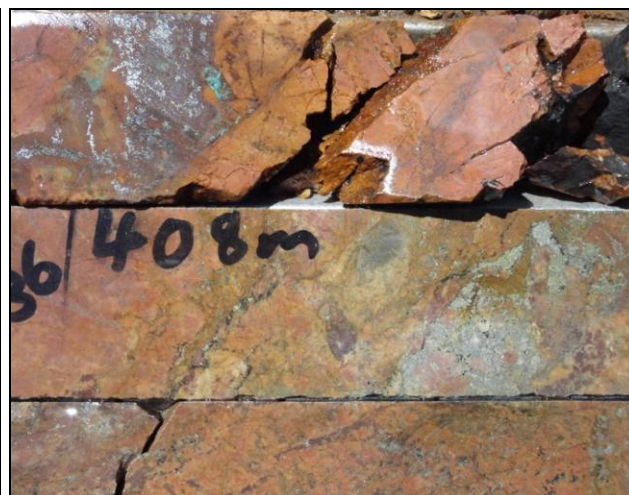
Secondary chalcocite + malachite in oxidised syenite in contact with hypogene pyrite chalcopyrite in carbonate altered syenite (S36-033, ~408 m)
