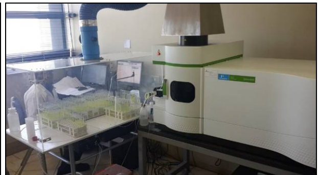
D) ICP-OES finish on ore grade digests
