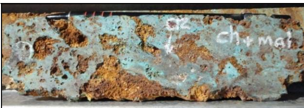
Malachite, pseudomalachite and chalcocite in weathered brecciated syenite (S36-033, 206 m)
