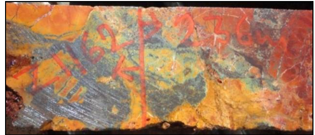
Chalcocite cemented breccia within high-grade supergene zone (S36-038, 236 m)
