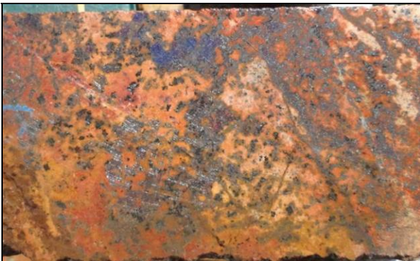
Fracture-hosted + disseminated chalcocite + bornite (S36-038, 236 m)
