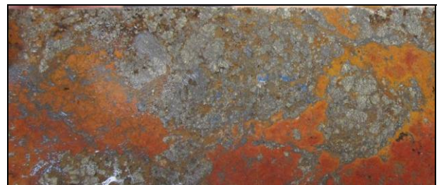
Remnant pyrite surrounded by digenite chalcocite and limonite, (KITDD_005, 310 m)
