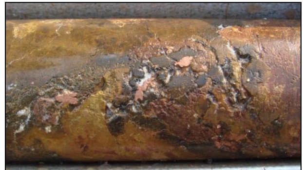
Native copper and calcite in vugs, hematite breccia (S36-015)
