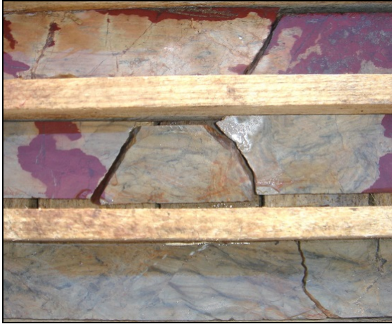
A) Steeply dipping and ripple cross laminated metasiltsone, with incipient brecciation, hematite alteration and pyrite mineralisation
