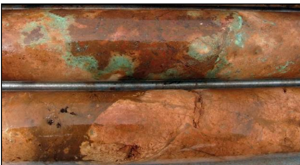
Malachite and pseudomalachite along fractures in quartz porphyry granite (S36-001; 126 m)
