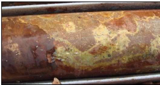
A) Pervasive K-feldspar alteration of syenite (KITDD_009)
