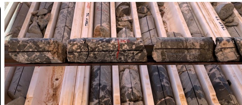
Above: NQ2 core from diamond drillhole 20ALDD0003 showing typical brecciation at approximately 365m downhole 1
