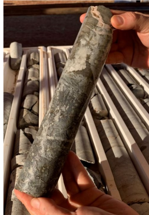
Above: NQ2 core from diamond drillhole 20ALDD0003 showing typical brecciation at approximately 365m downhole 1
