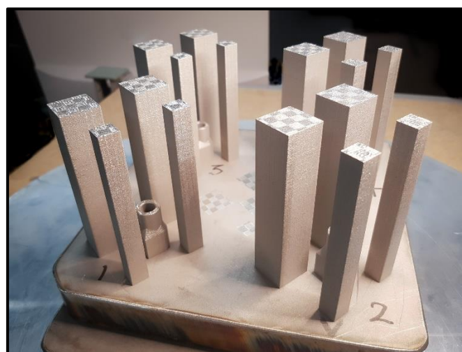
Fig 2: Tensile Bars printed at high laser power
