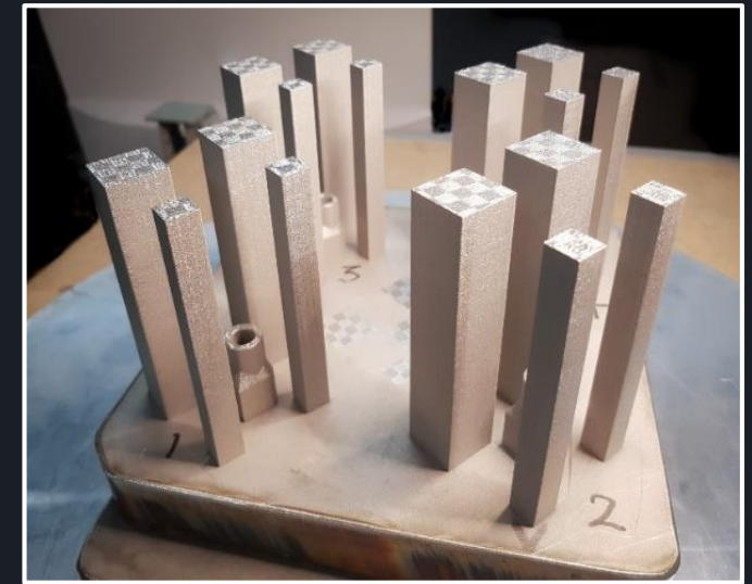
Tensile bars printed in 316L Stainless Steel
