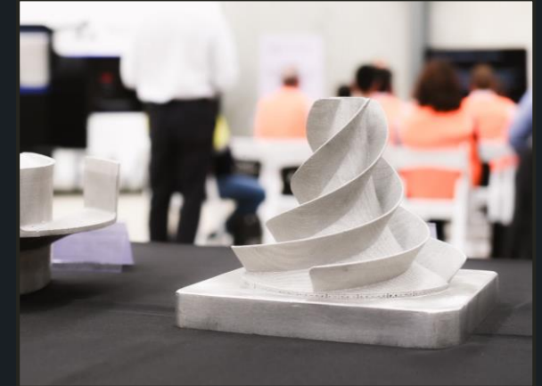
Hydro pulper printed in 316 stainless steel
