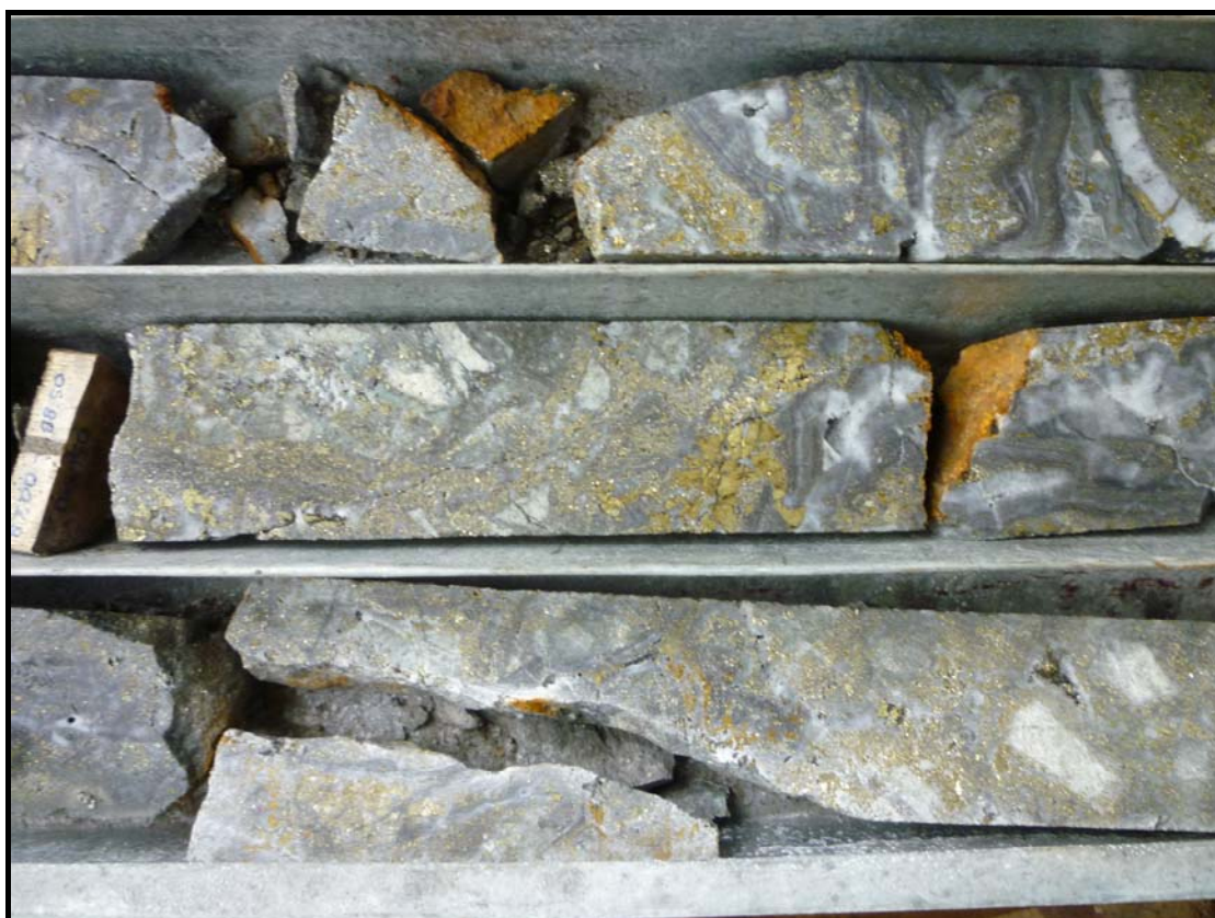
Drill core from hole JADD24 showing extensive copper mineralisation.
