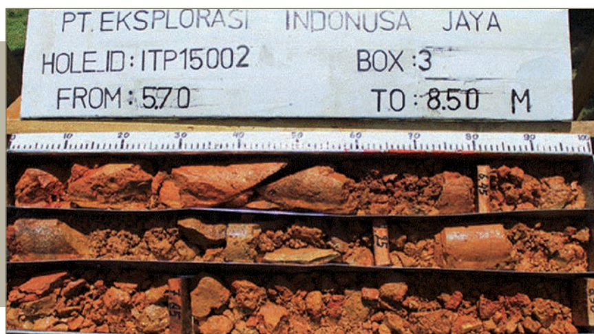
Drill core from Tapadaa drill hole ITP15002. Intensely oxidised vuggy quartz grading 0.63 g/t gold over the interval 5.0 to 9.0 metres is shown.
