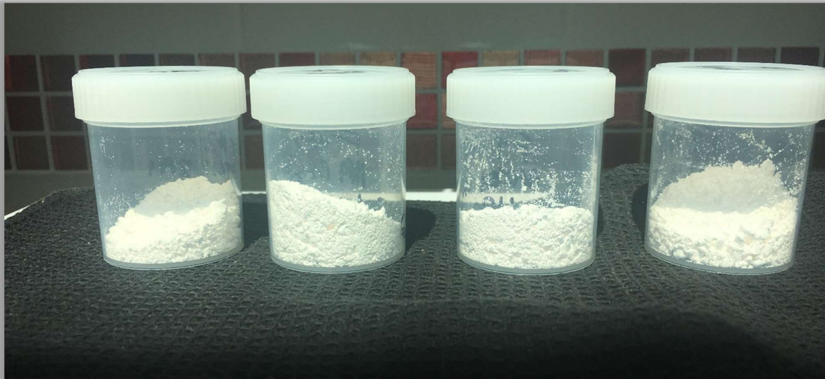
Figure 1: High Purity Alumina produced from the second SX mini-rig run
