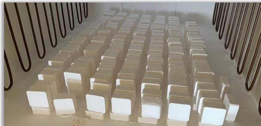
Sintering of HPA pellets for sapphire glass manufacture
