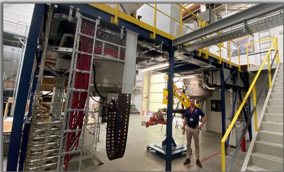
Twin set of sapphire growth units (Fametec Austria)
