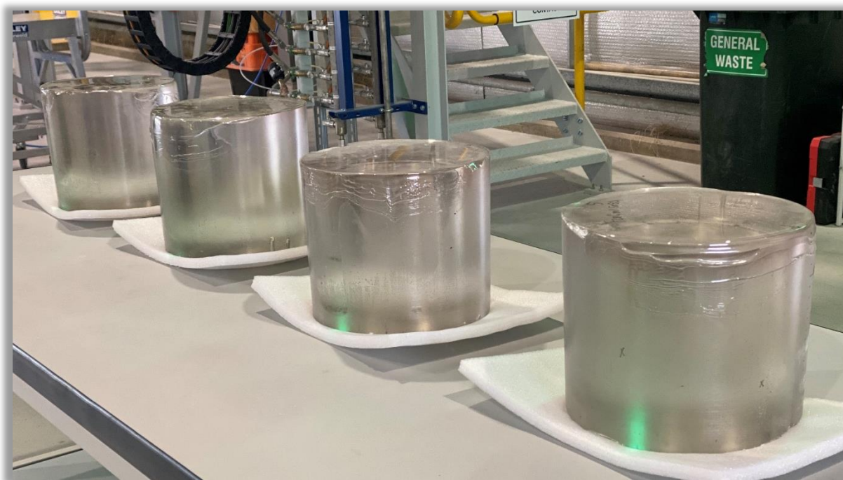
Successful sapphire boule growth from Phase A sapphire growth units
