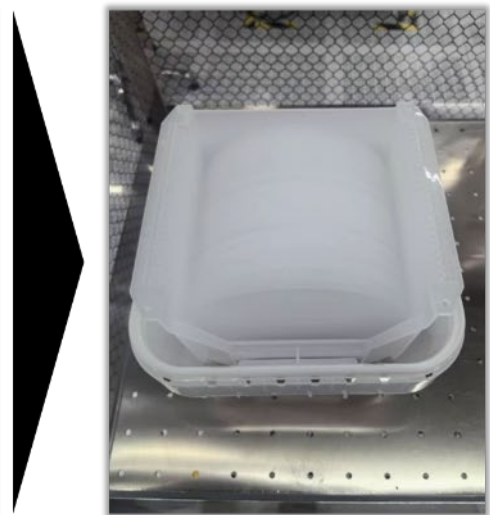
Successful sapphire boule growth from Phase A sapphire growth units (LHS) and cassette of completed 8" (200mm) sapphire wafers for GaN-on-sapphire semiconductor end-user (RHS)
