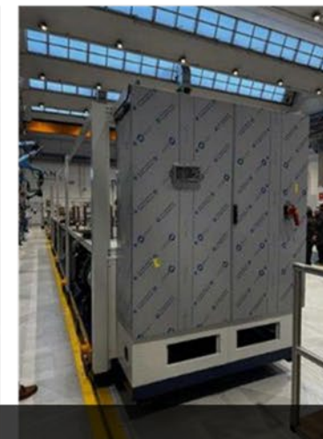
Water-chiller under fabrication
