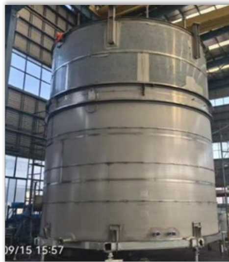
Completing trial assembly of large volume reagent and by-product tanks
