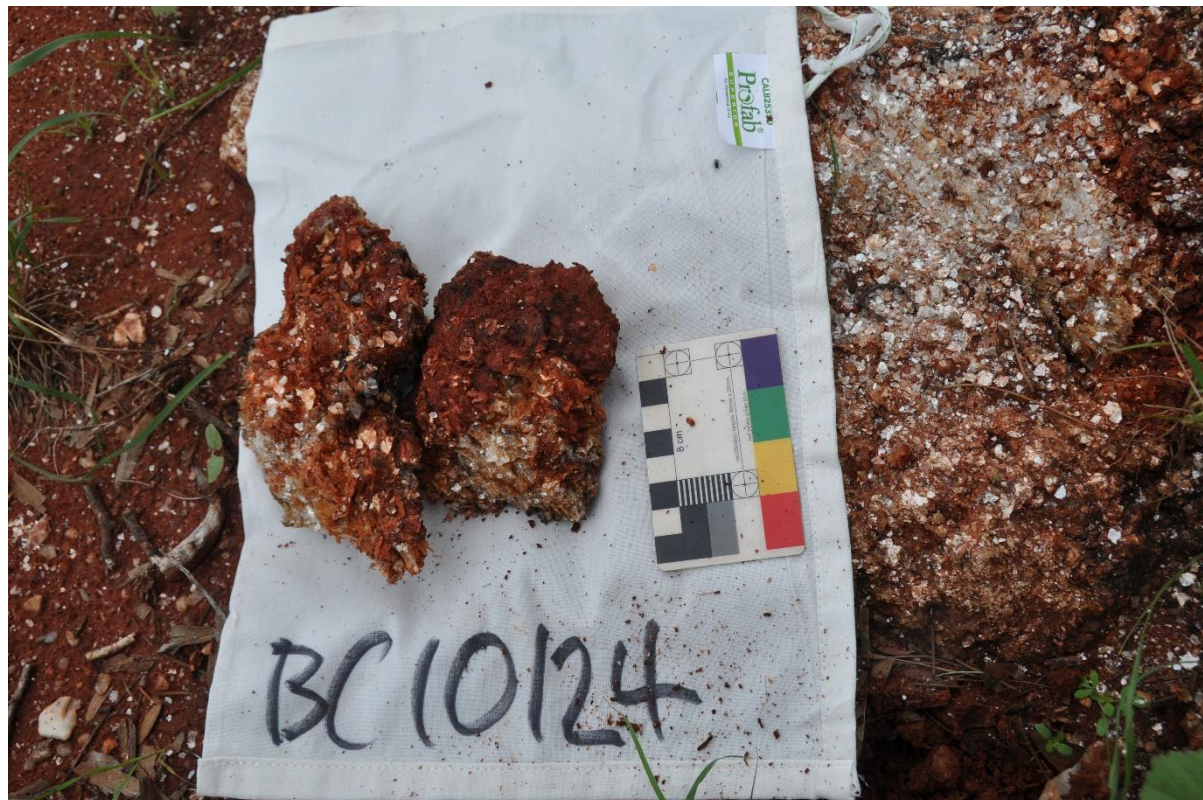
Figure 3: Sample BC10124, weathered mica-rich pegmatite with Ta reading up to 1018 ppm, Sn up to 640 ppm and Cs to 1911.9 ppm
