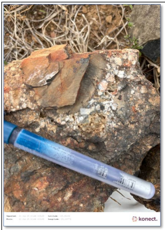
Photo 1: Breccia typically consists of sub-angular fragments of siltstone, possibly slightly altered in part.
