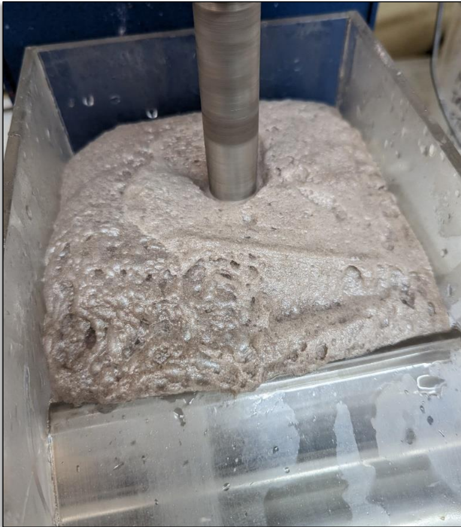
Figure 4: Mt Deans sample undergoing flotation test.
