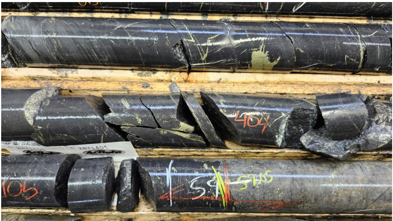
Photograph 2: Tillex Project TX26-005 Diamond Drilling Core, Mineralised Porphyry/Argillite Contact @59m Depth
