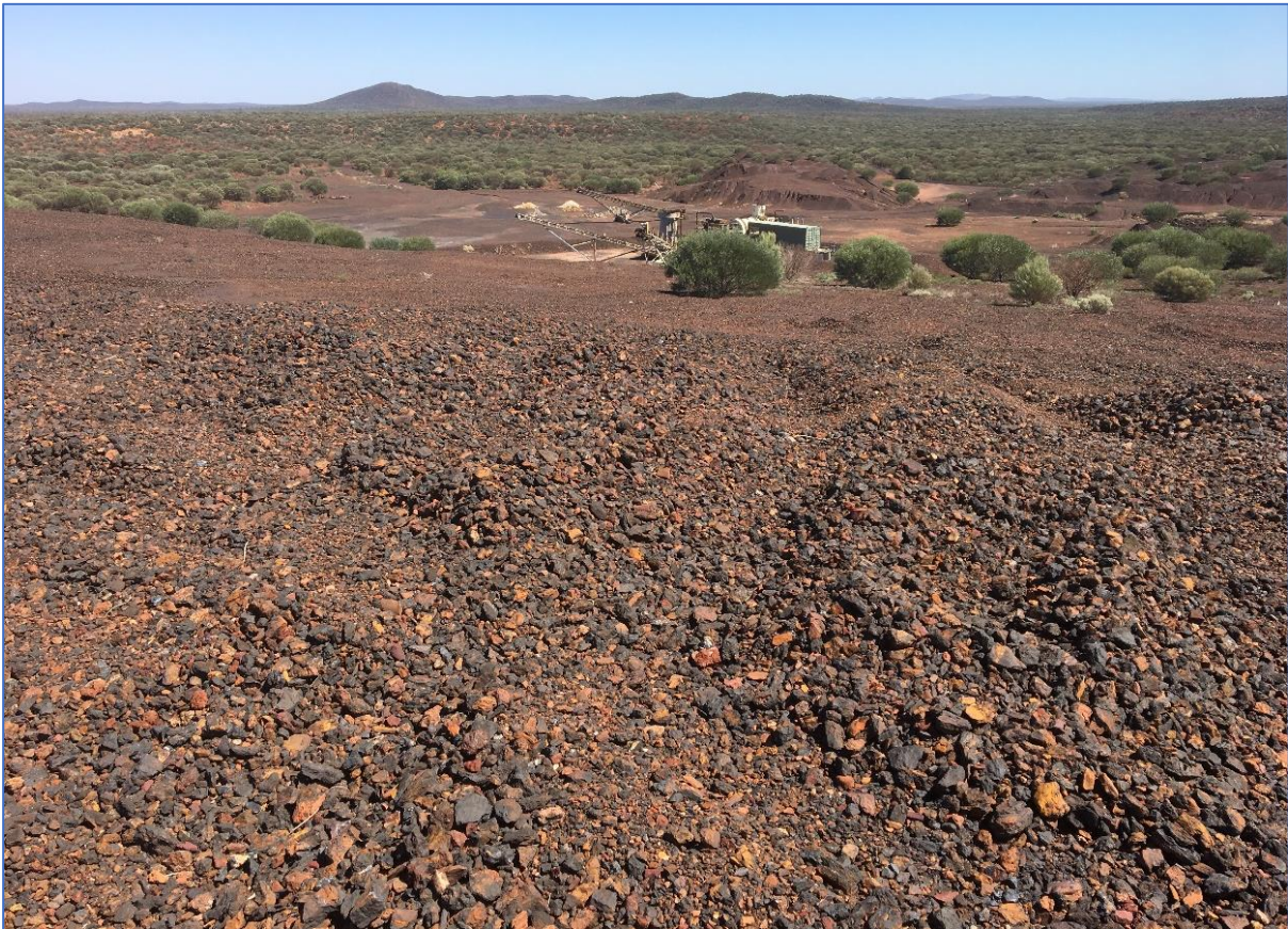
Plate 4 – View of Horseshoe South Mine taken from the top of the coarse sub-grade Mn stockpile (foreground), showing MIN’s beneficiation plant and fine sub-grade Mn stockpiles (background).
