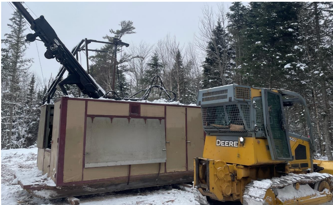
Figure 1 - Diamond Drilling at Bond Road Antimony Prospect
