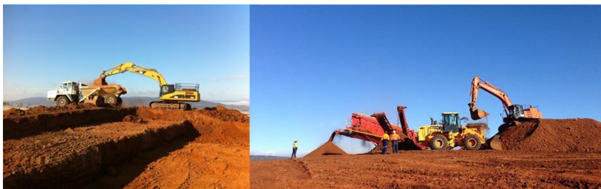
Figures 3 & 4: Bench mining pit MB3. Feeding dried ore to screen at MB5
