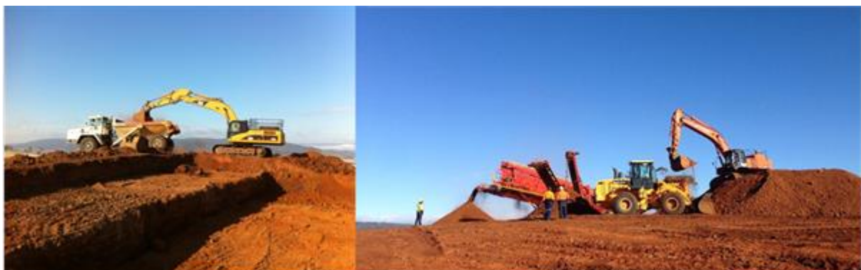
Figures 2 & 3: Bench mining & dry-screening by Stornoway Contractors
