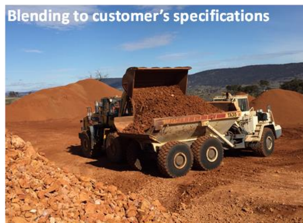
Figure 3: ABx supply chain operations from pit to mine stockpiles, blending, transport and stockpiling at Bell Bay Port.
