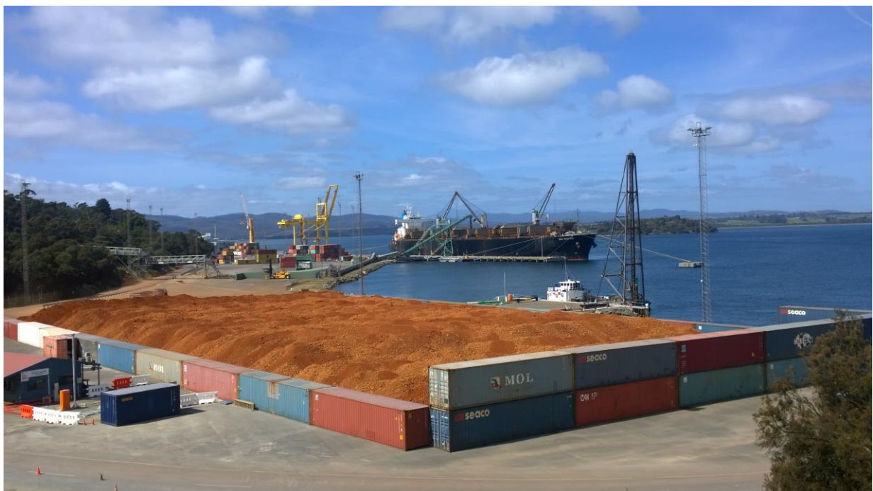
Figure 2: The 30,000 tonne cargo assembled at Bell Bay export ports. Note that the containers are used as dust barriers to prevent cross contamination with other cargoes. The bauxite is shipped in bulk carrier ships similar to the ship shown here.
