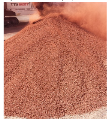
Figure 2: Screening of 28 tonnes of Binjour bauxite at Gympie
