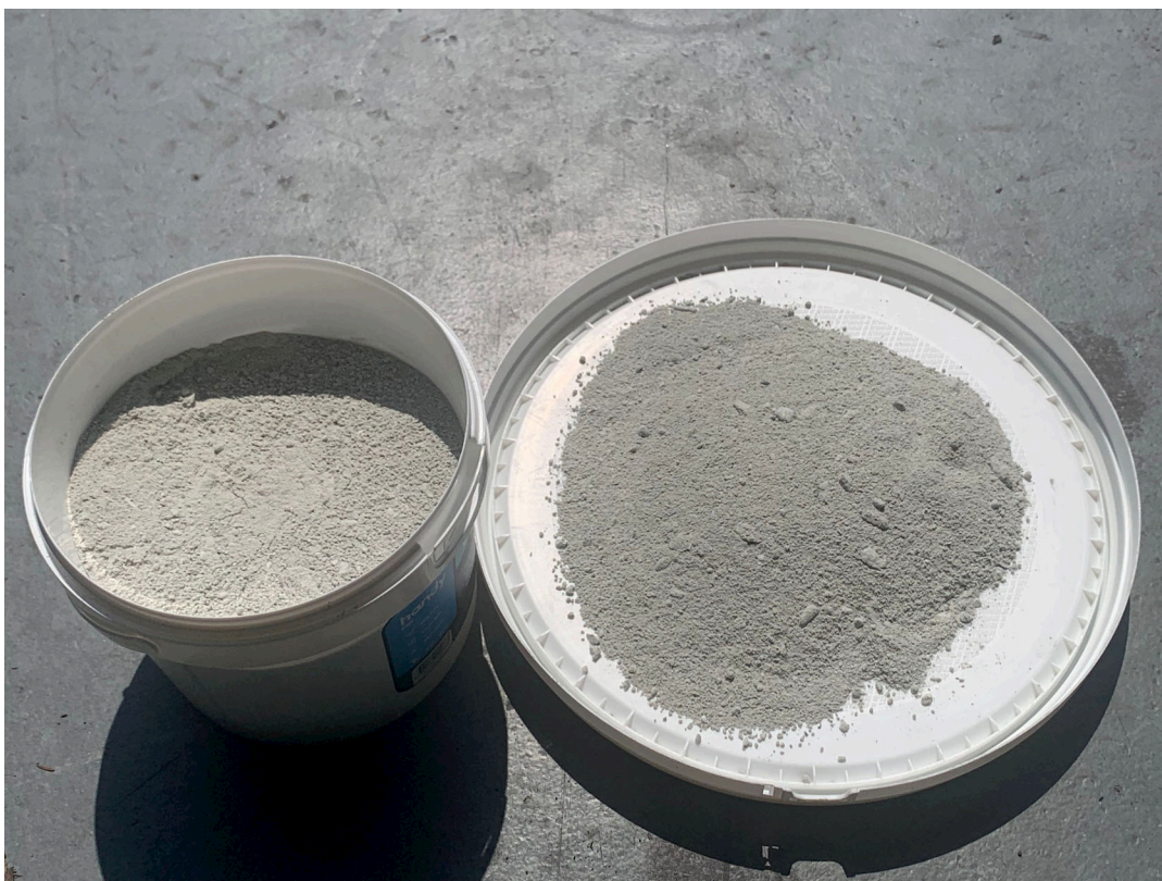
Figure 2: Sample of metal sulfate powder produced from bath pilot batch reactor.
