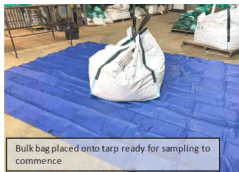
Figure 5 (left): handling the bulk sample from the pit, Preparations for drying the 183.7kg bulk sample in 42 trays
