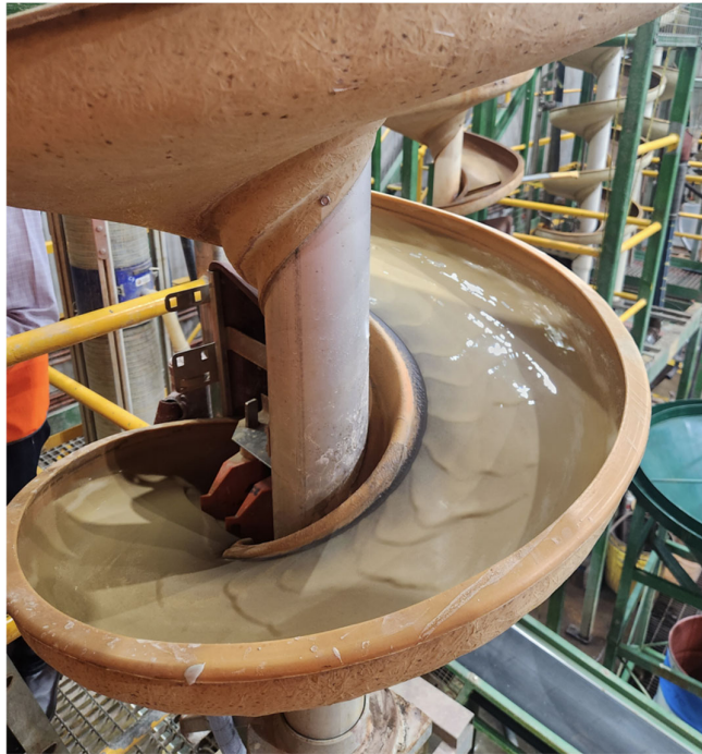
Figure 8 – Wet Spirals separation.
