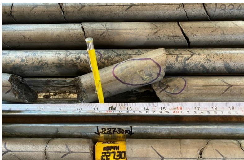
Figure 1 Massive sulphide unit of 4.15m showing sulphide composition and chalcopyrite blebs
