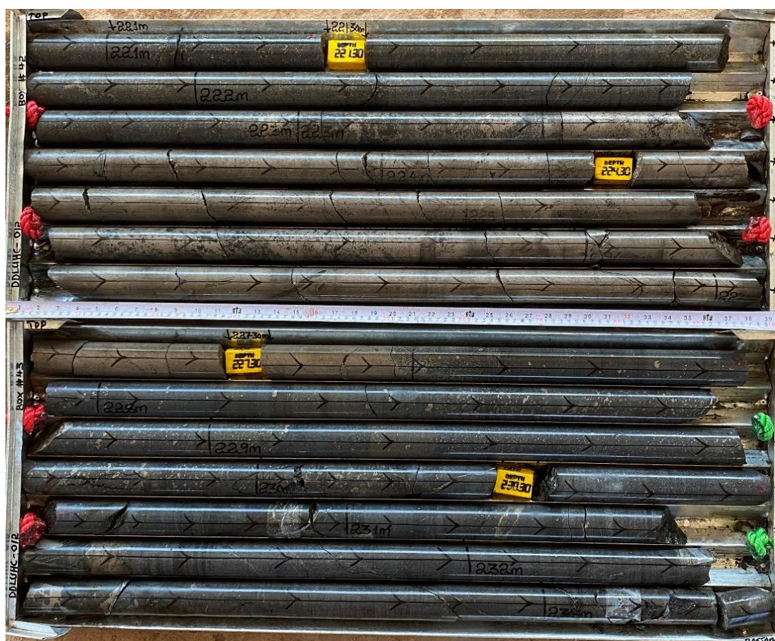
Figure 3 Core photo of the visual mineral intercept zones in DDLUHC001 at Luhuma Central of 4.15 metres of nickel bearing massive sulphides between 223.35m and 227.50m down-hole
