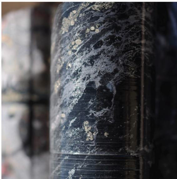
Plate 3 Drill hole WGR1D049-2 (~587m down hole): Silver-grey bismuth sulphide in chlorite rock.
