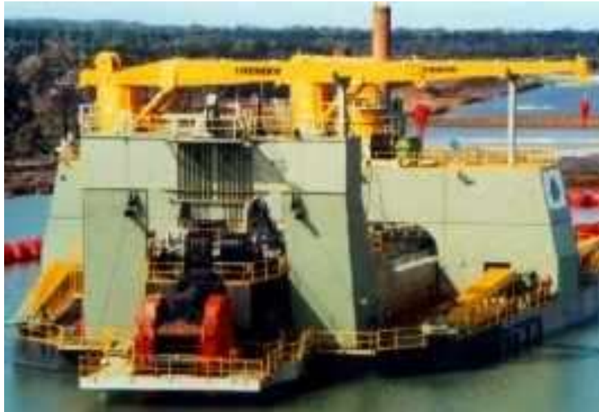
Figure 7 - Typical tin dredge
