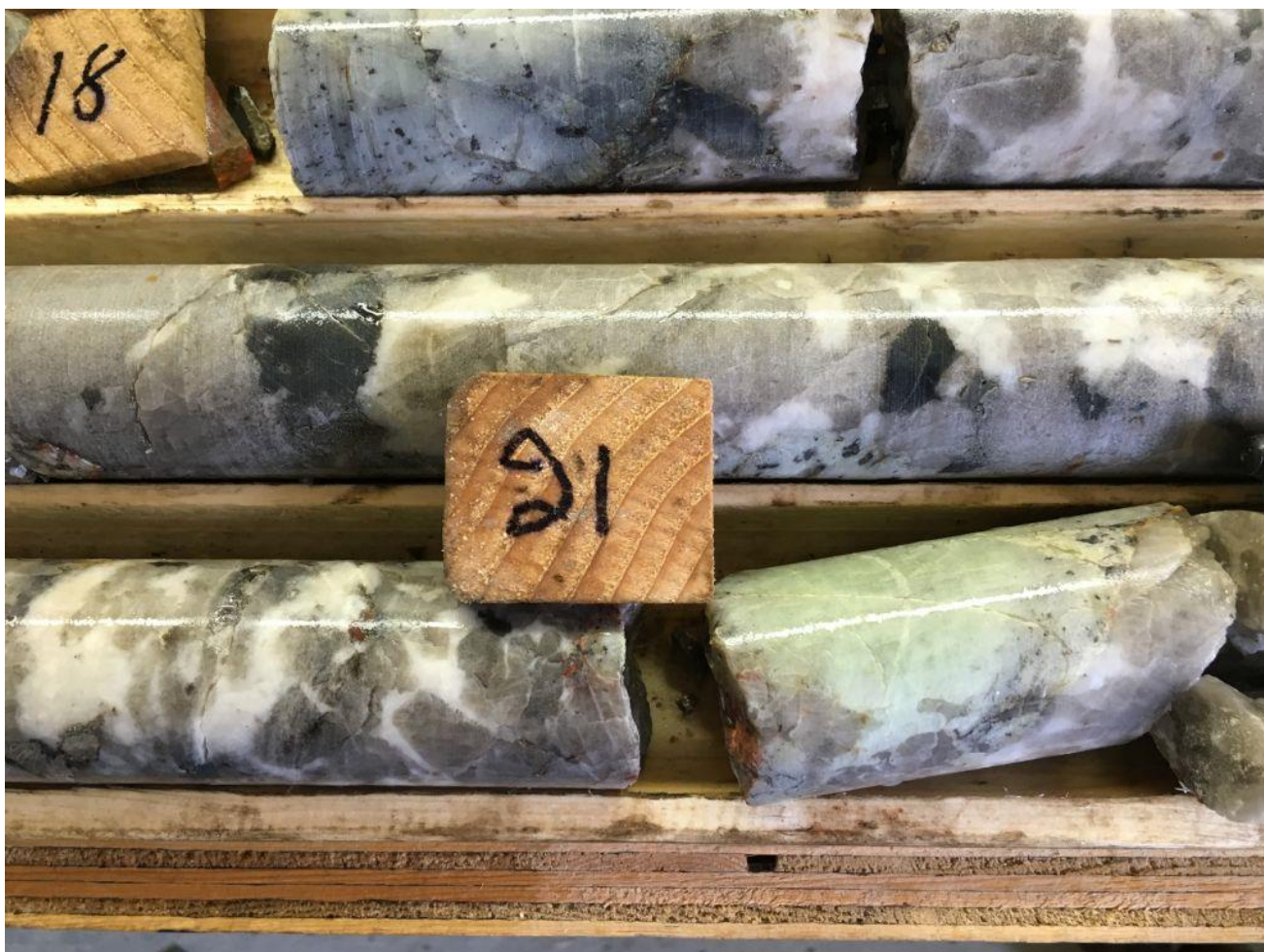
Figure 1: Photo of diamond drill core from hole SL-16-41 from Seymour Lake project showing the presence of the spodumene-bearing pegmatite.
