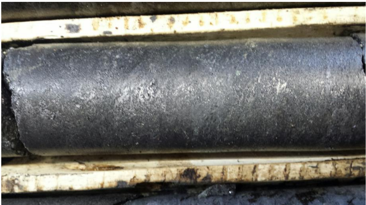
Figure 16: Graphite core from current drilling at Manitouwadge graphite project in Ontario, Canada (Hole EM 12-05 at Silver Star Prospect)
