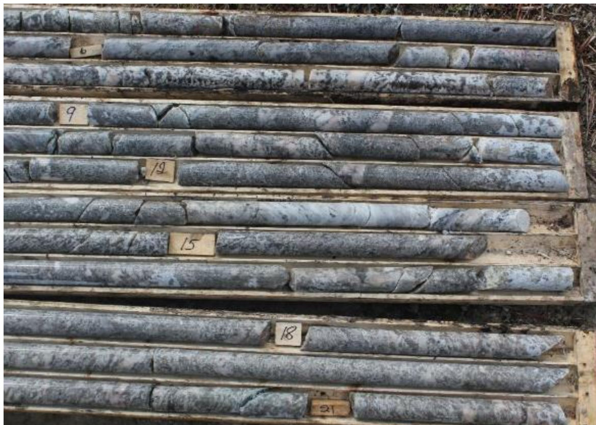
Figure 8. Drill core from the Root Lake Project showing multiple intersections of spodumene mineralisation in the pegmatite structures.
