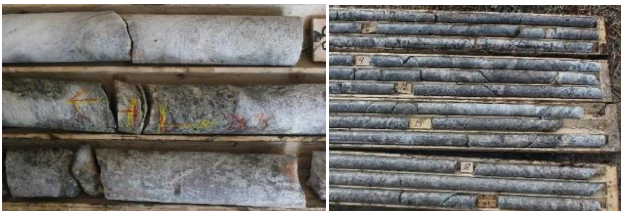
Figure 6. Drill Core from the Root Lake project showing multiple intersection of Spodumene mineralisation in the pegmatite structures.
