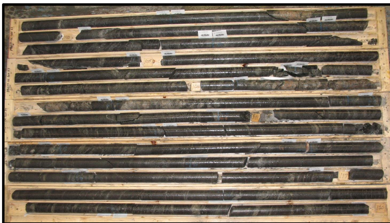
Figure 2. Drill core (MW-16-06) showing substantial graphite mineralisation.
