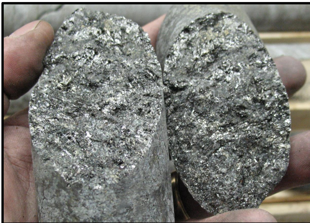
Figure 1. Drill core (MW-16-11) showing visible large graphite flakes
