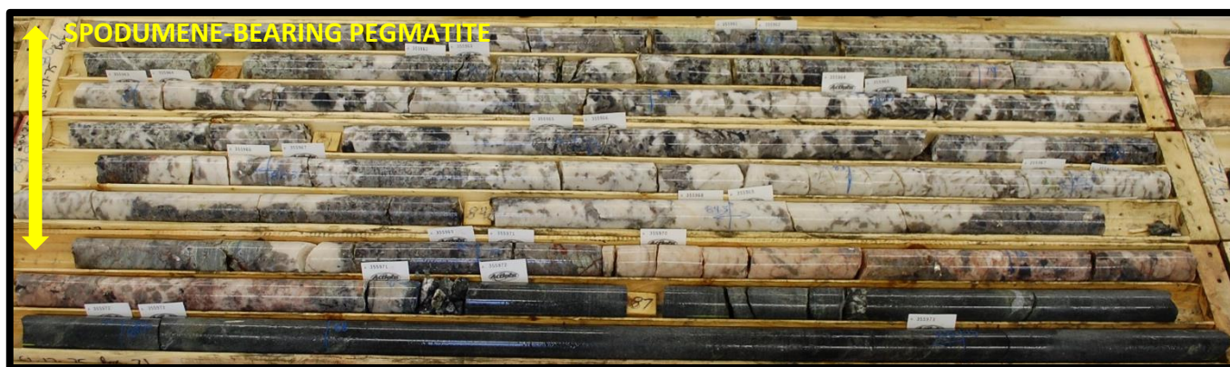
Figure 2. Drill core obtained from drill hole SL-17-75 (from 76.4.8m to 89.0m) showing the intersection of high-quality spodumene-bearing pegmatite (the lighter coloured material in the photo is the Pegmatite, whilst the darker material is Mafic Volcanic).
